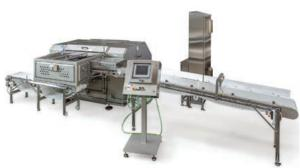
Danfotech bacon presses utilize a 3-dimensional press chamber to press bacon, philly steak, roast beef and other products to increase slicing yield and efficiencies. Danfotech's technology does not use a conventional hydraulic press in the system. This results in water savings because water is not needed to cool the conventional hydraulic operated press. Pacproinc Packaging Technology
